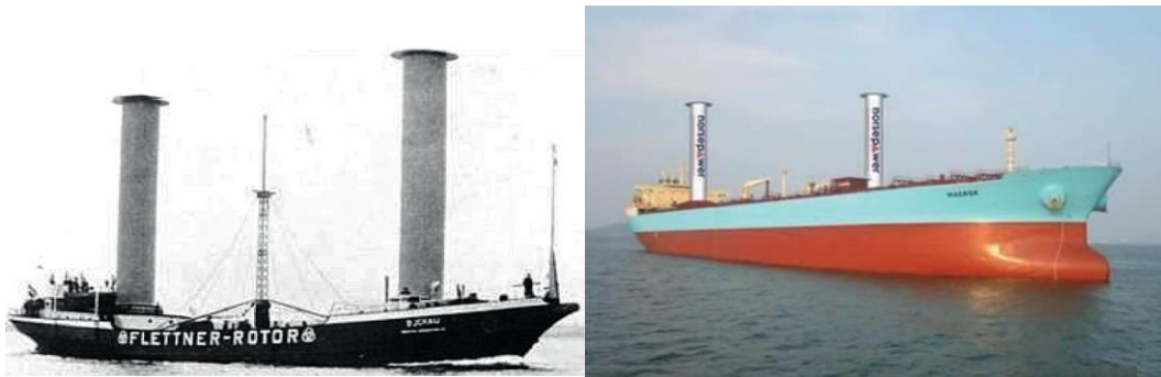
Figure 2.2: Applications of Flettner rotors on ships (Li et al., 2021; Tillig and Ringsberg, 2020).
