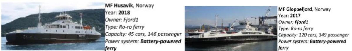
Figure 2.3: Electric passenger ferries currently in operation in Norway (Al-Falahi, 2019).
