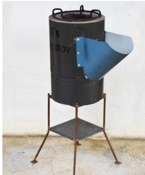
Figure 1: Efficient Stove often referred to as Rocket Stove 1
