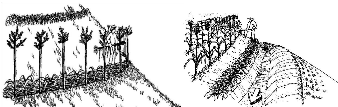
Figure 1: Structure of slow-forming terraces and contour ditches
