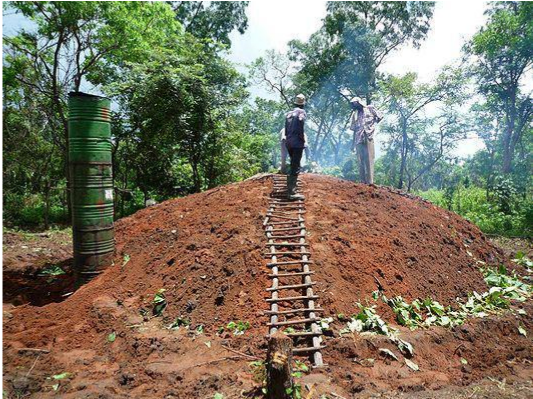
Figure 2: One of the improved charcoal production earth kiln in Malawi (Casamanance Kiln)
