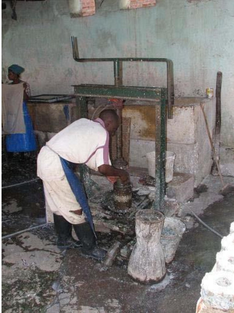
Figure 3 (b)3: The Screw-based presser used by non-profit organization Paper Making Education Trust (PAMET), based in central Blantyre (now not functioning)
