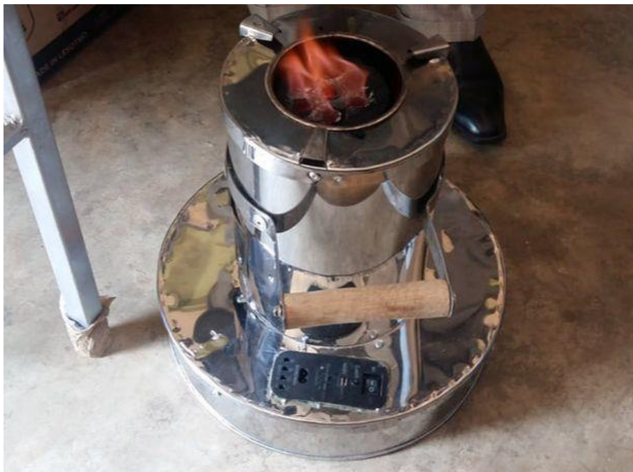
Figure 1: A Simple biomass gasifier cookstove
