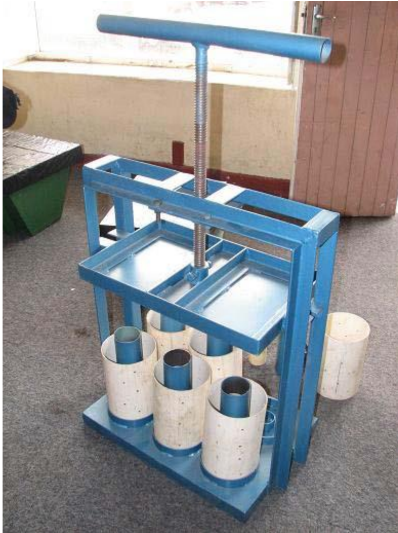
Figure 3 (a): The Screw-based presser produced by Malawi Industrial Research and Technology Development Centre (MIRTDC)
