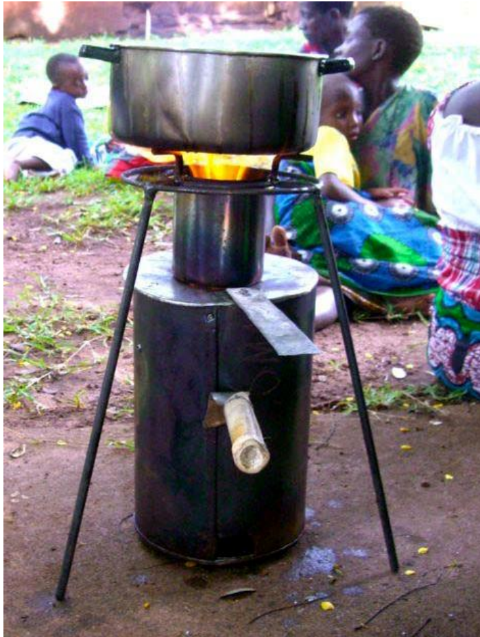
Figure 1: A Simple biomass gasifier cookstove
