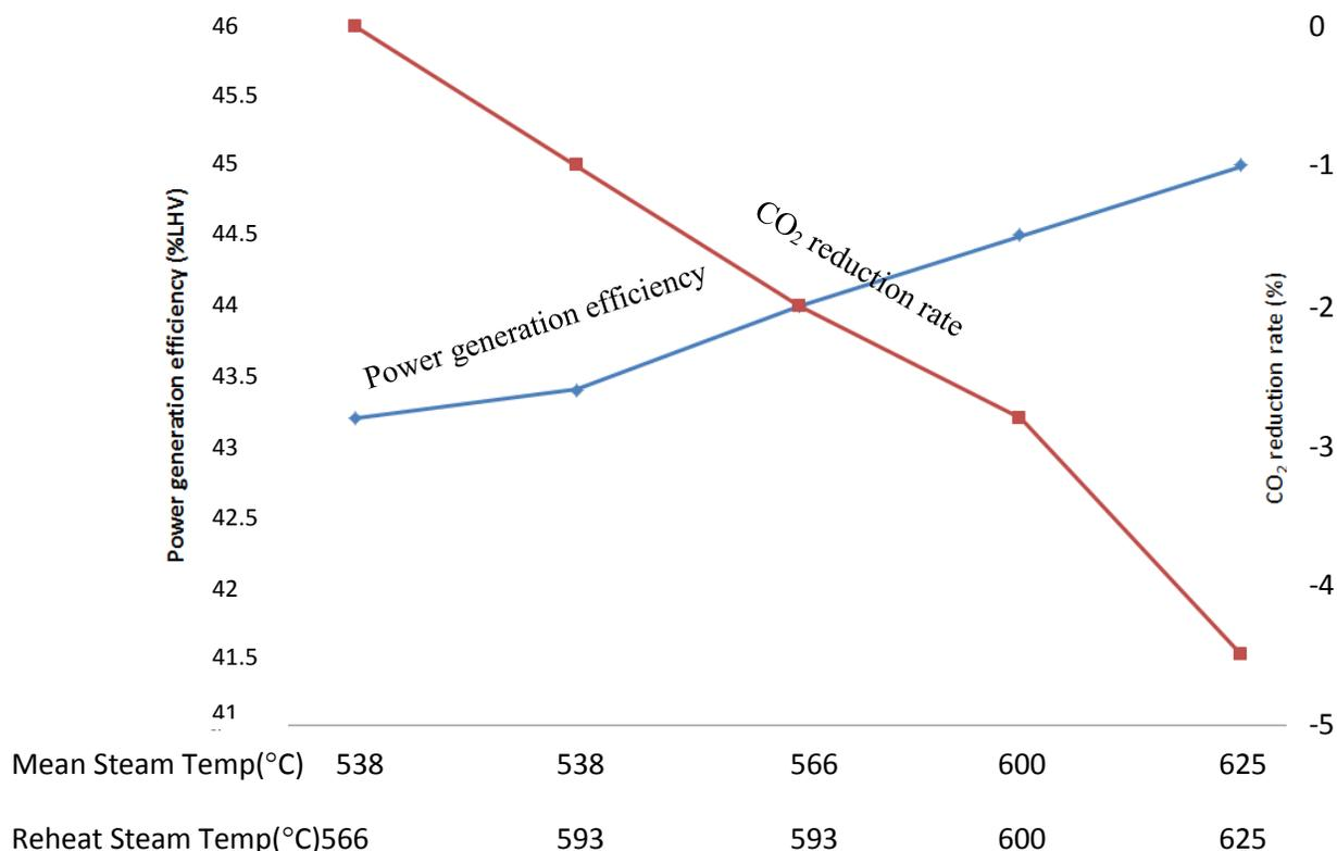
**Fig. 2 Power generation efficiency and CO<sub>2</sub> reduction rate for various steam conditions**
