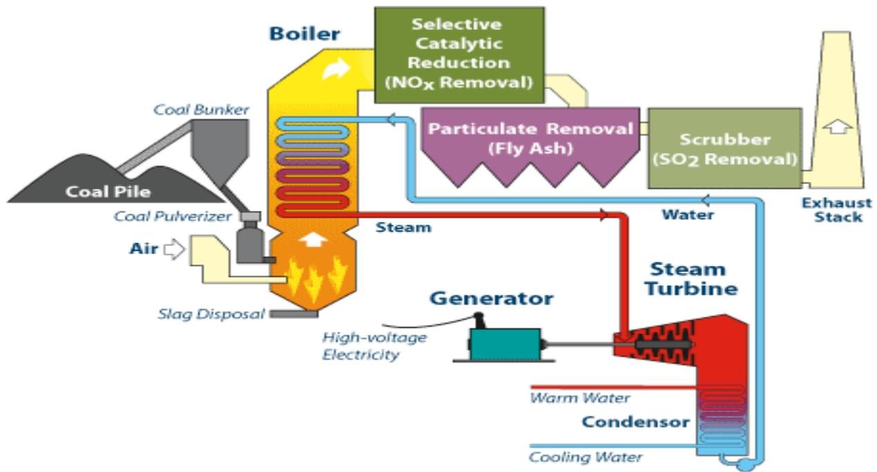
Fig. 1 Pulverized coal-fired power generation system (Rankine cycle)
