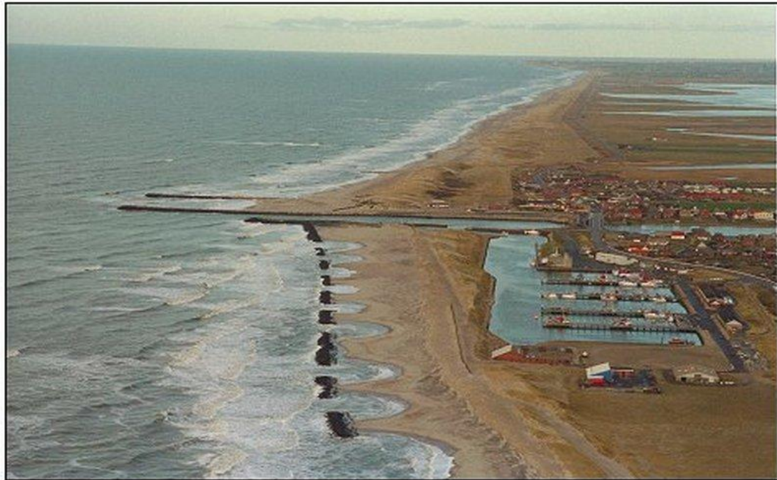
Photo 7. Artificial introduction of inert material with intermissions
